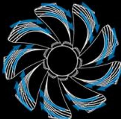
Focus air flow to optimize cooling efficiency
